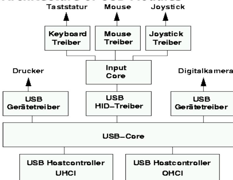
hid.o (HID = Human Interface Device) and input.o (Input Core) are only for a USB keyboard (usbkbd.o), Mouse (usbmouse.o) or Joystick otherwise they are not needed.
